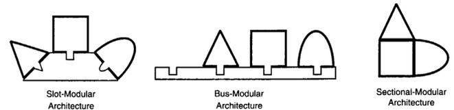
**Figure 1** Types of Modularity
